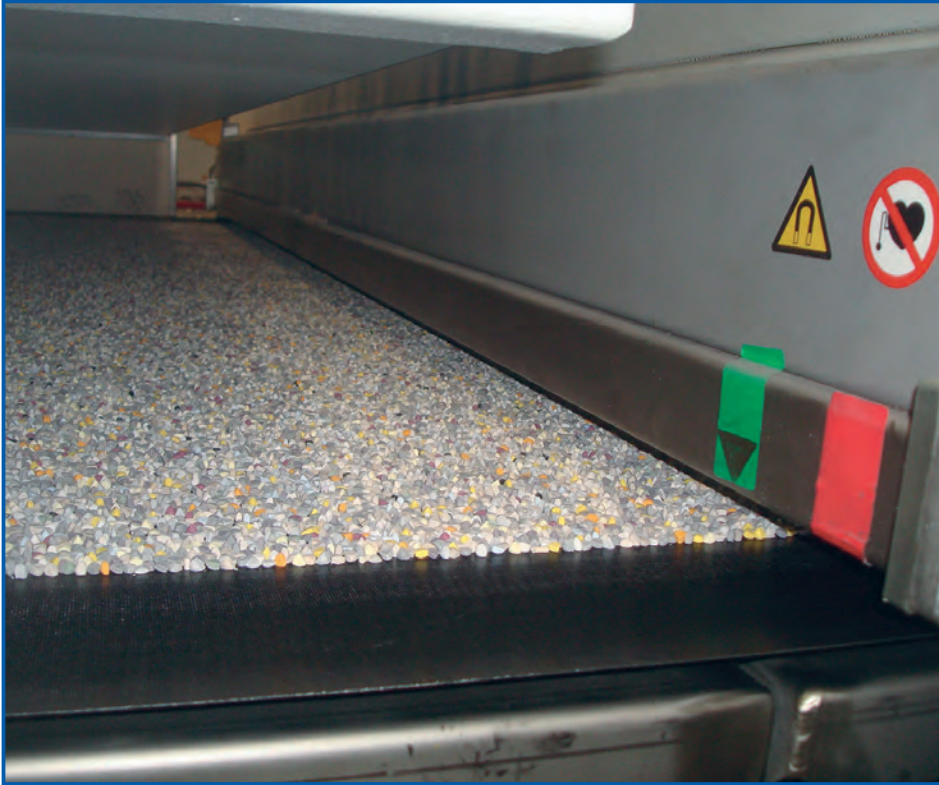
Scattered Vinyl granules on their passage to the heating zone, the press and the cooling zone
