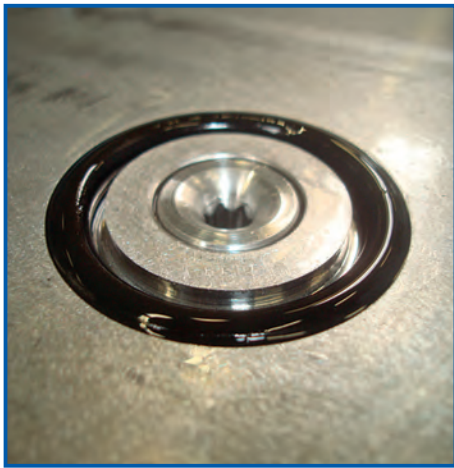
Figure 1. Former Al-nozzle and standard O-ring in a Hydro-Dyn press
