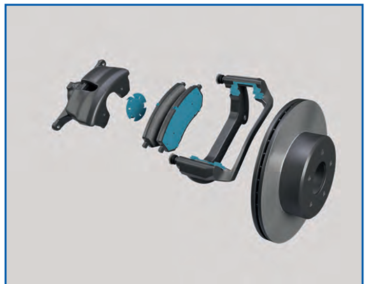
Exploded view of brake in a car showing the position of the brake shim
