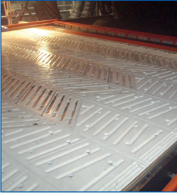
Figure 11. New design Teflon edge pads improving the product edge quality
