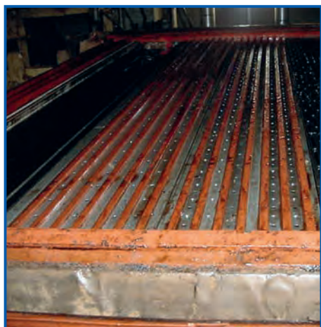
Hydro-Dyn press with 2 scraper pads at the top and bottom in the press out-feed area
