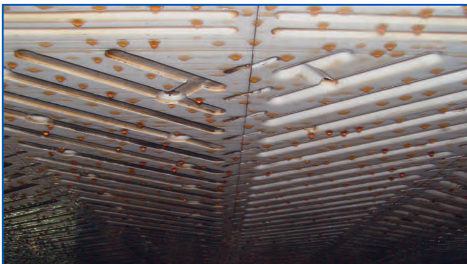
Both Teflon pad types in the press after 3 years of operation in the machine
