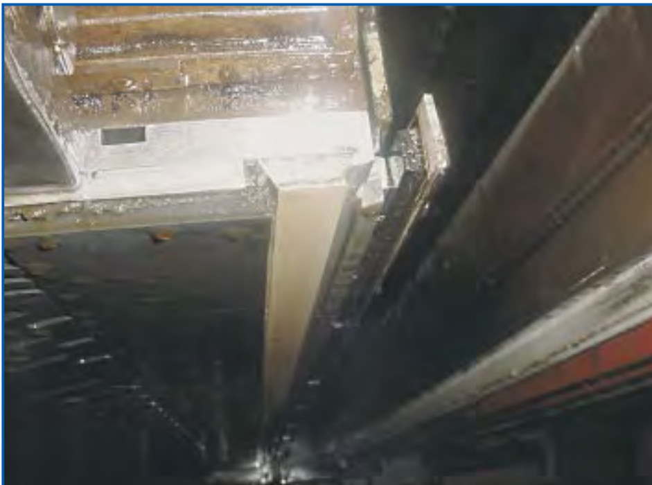
New press infeed with lower PEEK ledge and contact bar
