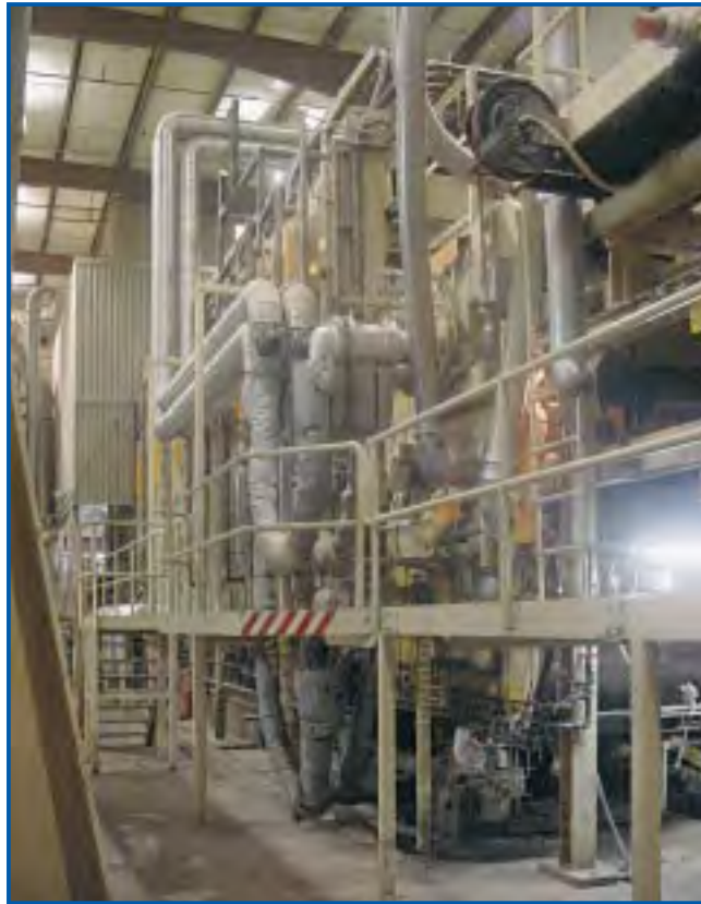
Press infeed of Flakeboard's thin MDF-press Fibrex II
