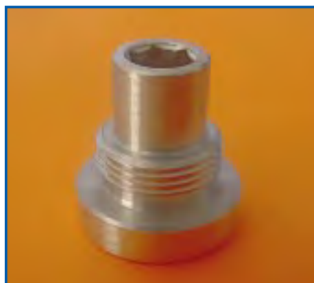
Modified Al-nozzle with new thread
